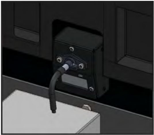
Correctly installed photocell Boiler ready for operation
